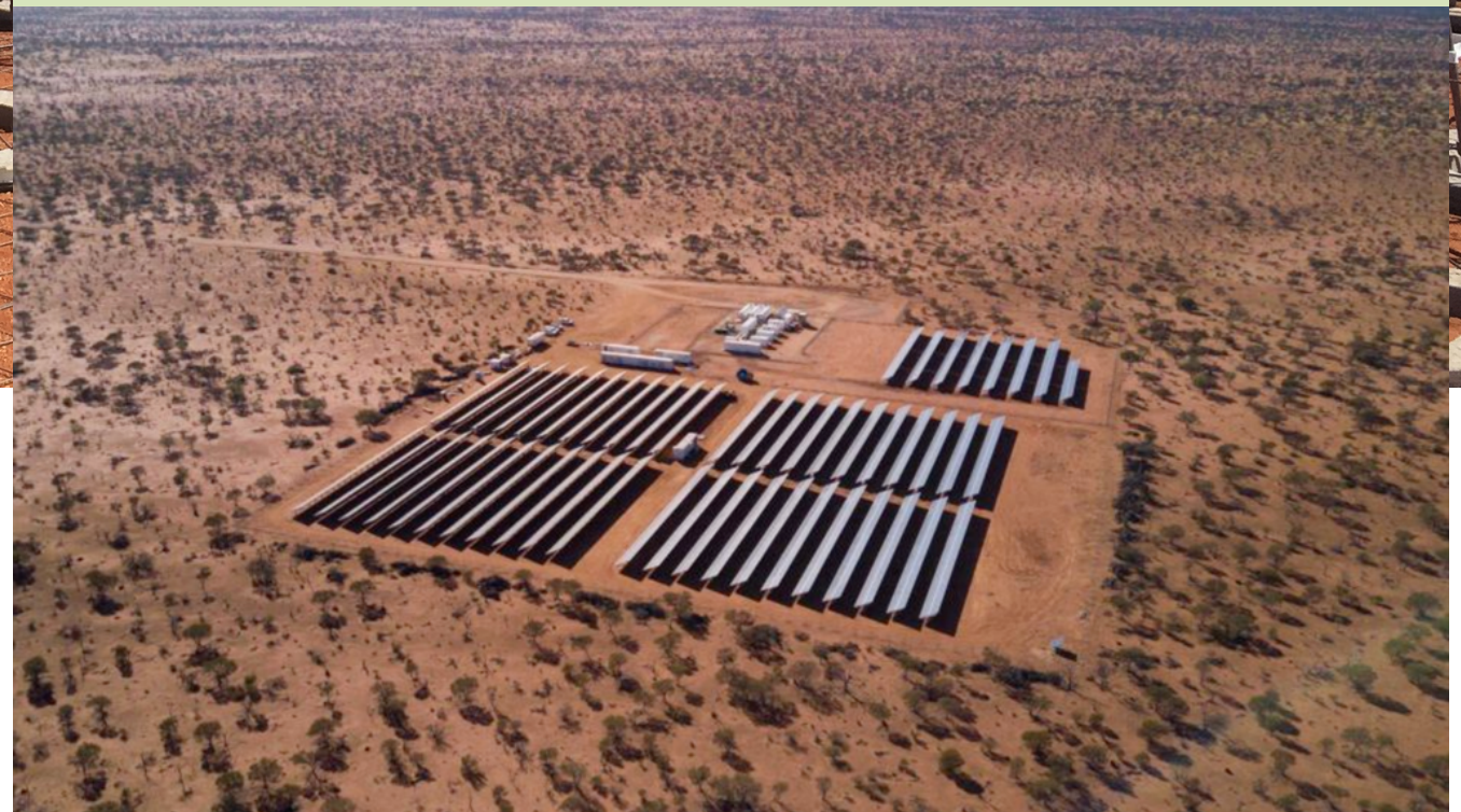
Solar power station: 2.6 MW-hr Lithium-ion battery
