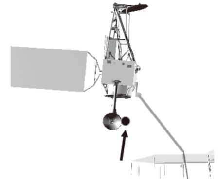
Figure 2. Developed retroreflector array optimized for the Astro-G's highly-elliptical orbit. The inner pyramid-shaped array for the low altitude supports wide range of incident angles. Outer surrounding flat retroreflectors for the high altitude contribute to increase the effective aperture area.
