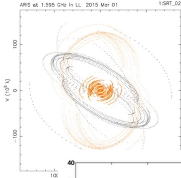
Simulated a L-band dual space-craft with multi-beam capabilities
