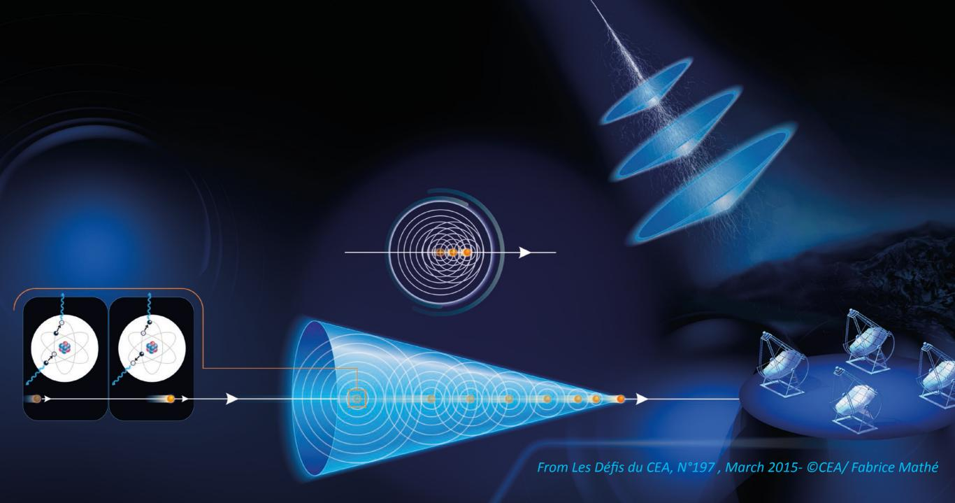
Using Cherenkov radiation from particles in extensive air showers to detect gamma and cosmic rays in the atmosphere
