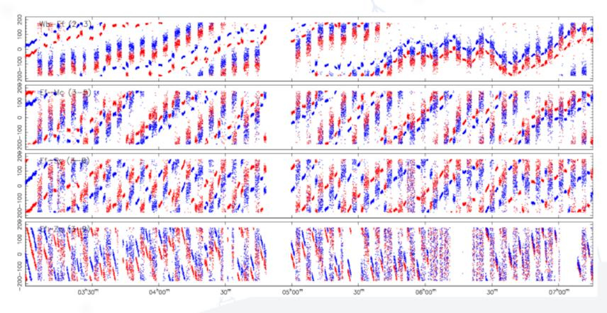
Point-like source at the phase center (phases should be zero!)
