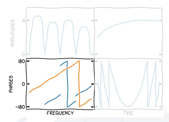
Multi-band delay (global fringe-fit) calibration
